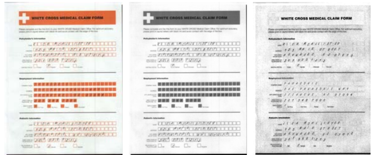
Left: Original form with color background for easier navigation. Middle: Form scanned in Monochrome mode without color dropout is hard to read and prone to image capture errors. Right: Form scanned using Color Dropout mode is now easy to read and delivers high image capture accuracy.
